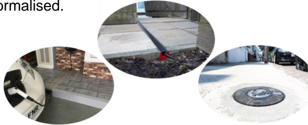
Figure 4 footway channelling, embedded and retractable solutions (Sources: Green Mole Ltd, Kerbo Charge Ltd & Trojan Energy )
