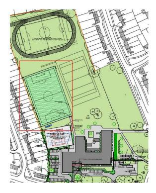
The MUGA would be surrounded by 4.5m high twin bar (weldmesh) fencing. It was originally proposed that this fencing would be topped with a 3.5m high ball stop netting making a total height of 8m. However, following adverse comments received from the Council's Landscape Consultant with regards to visual amenity, the ball stop netting has been removed. A 1.2m high Super Rebound Panel would be fixed to the bottom of the proposed fencing to help reduce the noise when balls hit the fence.
