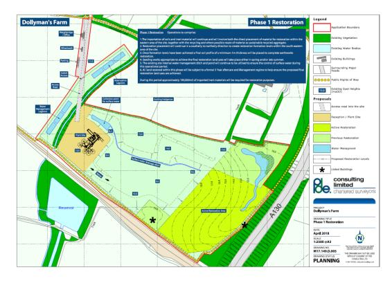
Phases two and three would see the importation and infilling continue in an east to west direction, with phase four (final restoration) seeing the decommission and removal of the plant site and reprofiling of this area, final shaping of water bodies and planting and the site restored to agricultural use with biodiversity enhancements.
