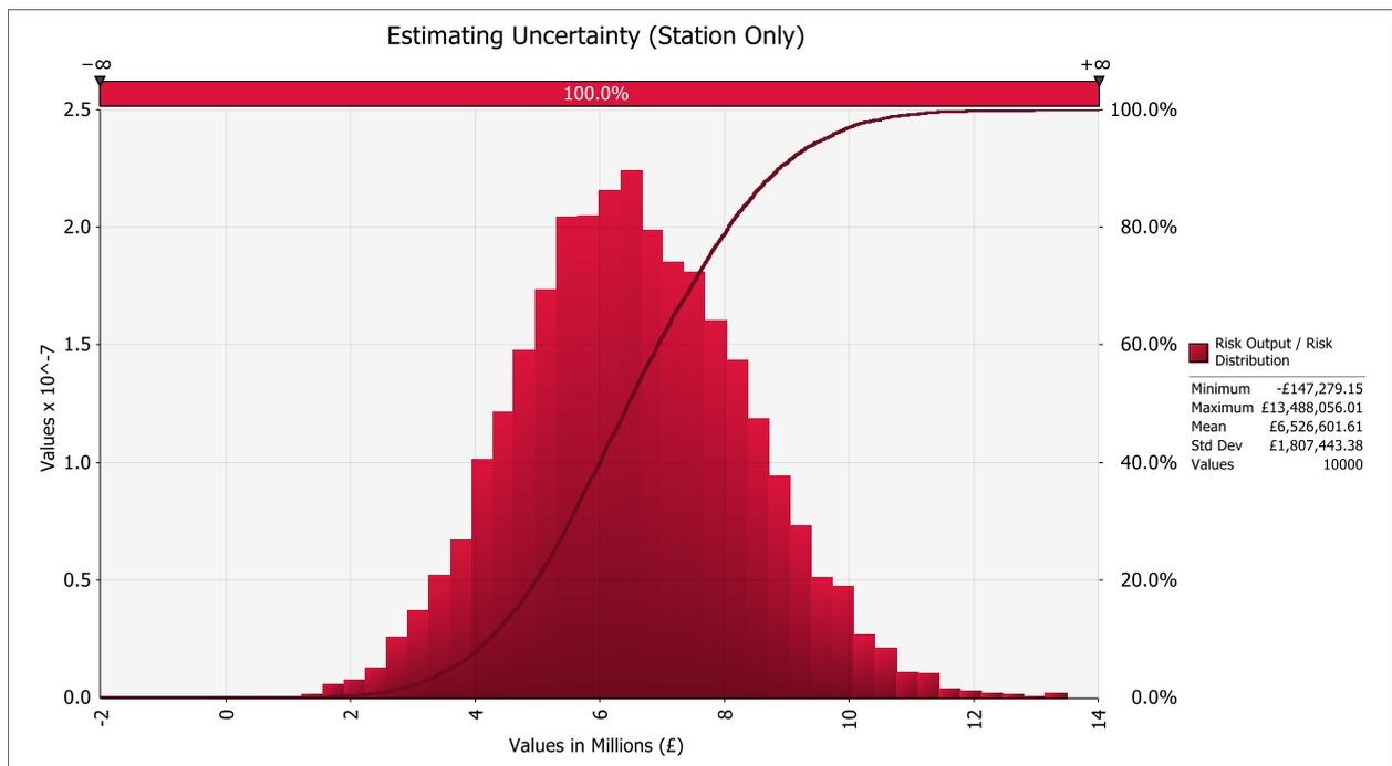
Figure 9.1 S-Curve showing estimating uncertainty for Station Only
