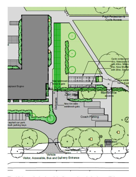
The Highway Authority originally questioned whether sufficient space would be available to provide access for emergency vehicles. Following the provision of a vehicle tracking drawing by the applicant which demonstrated access for emergency vehicles could be provided, the Highway Authority raised no objection to the proposal.
