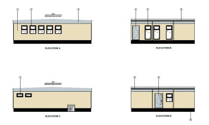
The building is of mainly timber construction which is a renewable resource. The building has LED lighting throughout, PIR controlled lighting (motion sensor lighting) to the main areas with daylight dimming and a heat pump system to provide the heating within the building. The building is insulated to achieve the elemental u-value standards (measure of heat loss in a building such as a wall, floor or roof) set out in Building Regulations.
