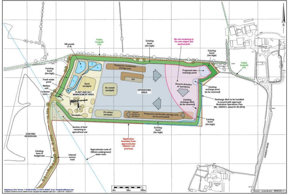
Sewells Reservoir Construction Illustrative Operations Plan Scale - 1:2,500 (at A3) Date - 02-12-2021 Plan No. 1003/O/2
